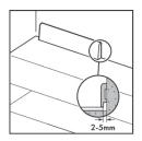
For standard residential use (15-35°C), the maximum room size is 13mx13m. For rooms with more extreme temperatures (5-65°C), the maximum room size is 8mx8m. For rooms with HVAC-system (18-25°C), the maximum room size is 30mx30m.
